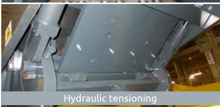
Hydraulic gap adjustment to prevent clogging
