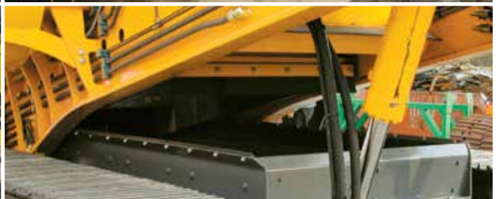
Patented hydraulic lifted chassis
