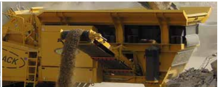
Separate driven pre screen
