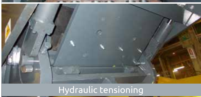
Hydraulic gap adjustment to prevent clogging
