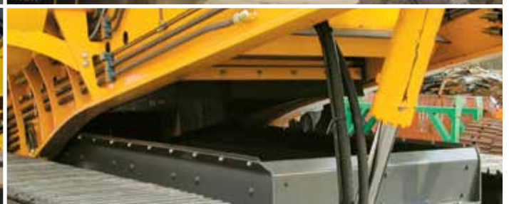
Patented hydraulic lifted chassis
