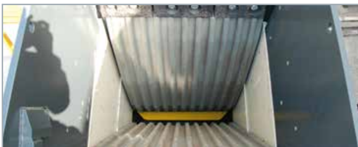
Hydraulic gap adjustment to prevent clogging
