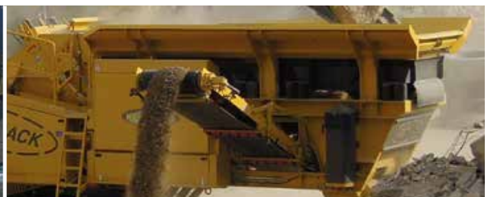
Separate driven pre screen
