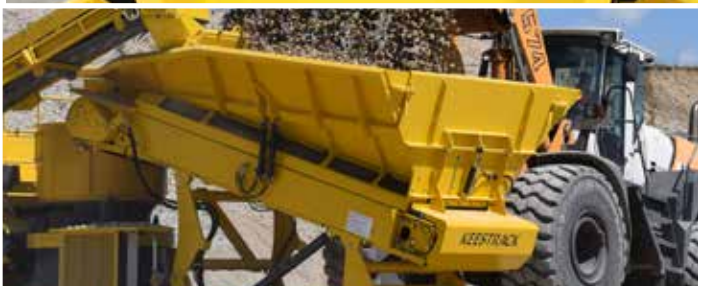
Hydraulic folding hopper walls
