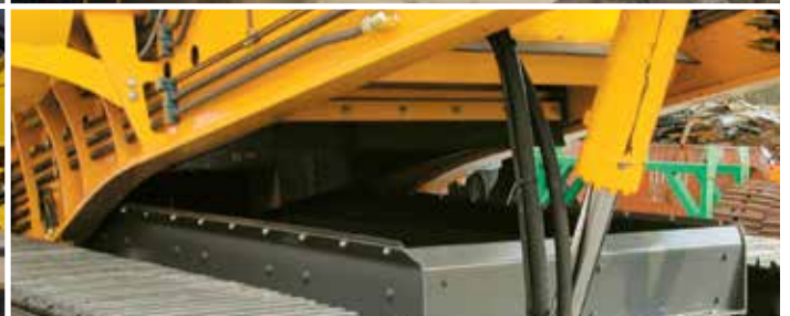
Patented hydraulic lifted chassis
