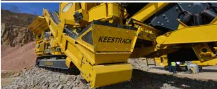
Swiveling return/stockpile conveyor
